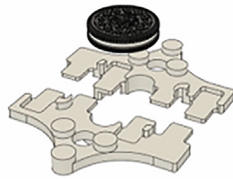
FIG. 11. This computer-rendered animation shows the assembly and use of our Oreometer including inserting the Oreo cookie into the two halves of the clamping fixture, inserting this fixture into the base, and adjusting the base separation, adding “penny castles” to the wings, adding pennies, and finally observing the fractured Oreo. Multimedia view: https://doi.org/10.1063/5.0085362.1
