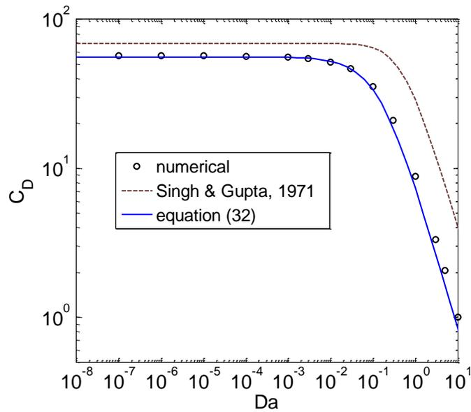
Figure 12: Drag coefficient on a porous cylinder varying with Darcy number at a fixed Reynolds number  $Re_D = 0.1$ . Numerical results (symbols) are for  $L_r = 50$ , the analytical solution of Singh and Gupta (Singh
