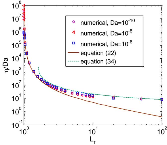
Figure 13: Scaled interception efficiency  $\eta/Da$  varying with plates spacing ratio  $L_r$  at  $Da = 10^{-10}$ ,  $10^{-8}$ ,  $10^{-6}$  and  $Re_D = 1$ : comparison of numerical data (symbols) with analytical limits for  $L_r \rightarrow 1$ , equation (22), and  $L_r \rightarrow \infty$ , equation (34).
