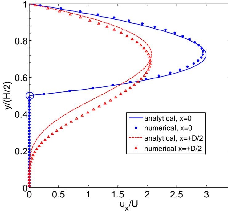
Figure 9: The  $x$ -component of the velocity in the gap at  $x = 0$  and  $x = \pm D/2$  from analytical solution (lines) for flow around solid cylinder and numerical solution (symbols) for flow past a porous cylinder with  $Da < 10^{-4}$ . In both cases,  $Re_H = 0.5$ ,  $L_r = 2$ . The hollow circle at  $y/(H/2) = 0.5$  indicates the velocity at the interface of the porous cylinder and the side channel at  $x = 0$ .
