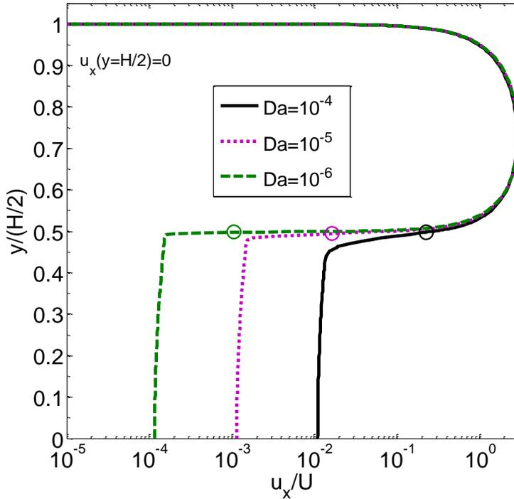
Figure 8. The velocity profile inside and outside the porous cylinder at  $x = 0$  obtained from the numerical solution at different Darcy numbers for  $L_r = H/D = 2$  and  $Re_H = 0.1$ . The hollow circle at  $y/(H/2) = 0.5$  indicates the velocity at the interface of the porous cylinder and the side channel.
