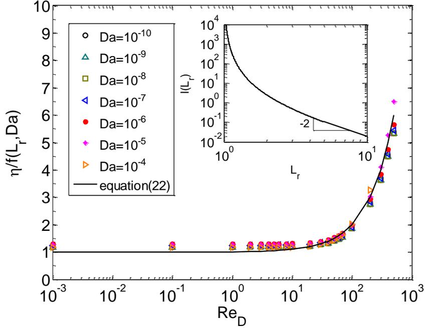
Figure 10: Interception efficiency varying with Reynolds number: the computed results shown in Figure 6 collapse by combining the effect of the Darcy number and the plate relative separation using  $f(L_r, Da) = \eta_{Re \rightarrow 0}$  given in equation (21), the solid line is (22) with  $c = 0.01$ . The inset plot shows the function defined in equation (19), which is used to calculate  $f(L_r, Da)$ .
