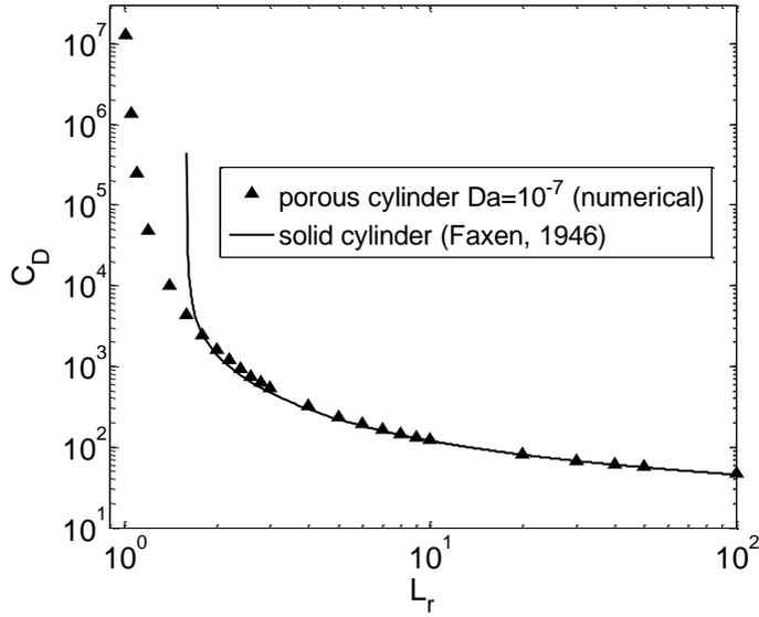
Figure 11: Variation in the drag coefficient of a porous cylinder with the plate separation ratio,  $L_r = H/D$  at  $Re_D = 0.1$ . Numerical data (symbols) are for a porous cylinder at  $Da = 10^{-7}$ . The solid line is Faxén's solution for a solid cylinder using the first four terms in the series expansion.
