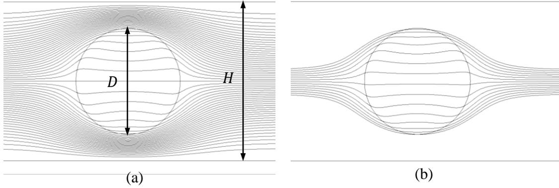
Figure 2: Concept of interception efficiency  $\eta = Q_c/(UD)$  shown with streamlines in flow past a porous cylinder between parallel plates (a) evenly spaced streamlines representing the total flow rate  $Q_{\text{tot}} = UH$  (b) isolating just the streamlines that intercept the cylinder, representing  $Q_c = U_a D$
