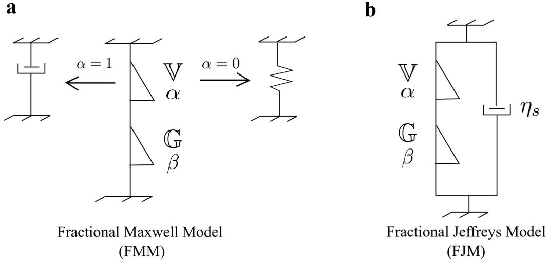
Figure 1: Schematic representation of the fractional Maxwell model (FMM) as two ‘springpots’ in series and the definition of a springpot as a mechanical element that interpolates between a spring ( $\alpha = 0$ ) and a dashpot ( $\alpha = 1$ ). (b) Fractional Jeffreys model (FJM) with two springpots in series arranged in parallel with a purely viscous (dashpot) element to account for solvent viscosity.
